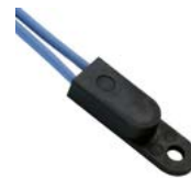
G-TD-THM01-006 80" Thermistor temperature probe with self adhesive patch. Temperature range of -80°C to 120°C. Compatible with our AA1 sensor interface.
