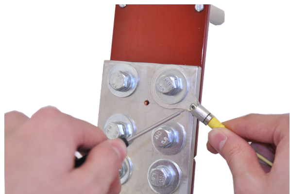
Figure 14: Secure Probe by Tightening Allen Key
